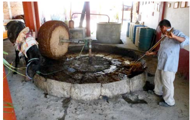
Burro-power drives a stone wheel that grinds roasted agave cabezas into pulp and liquid for subsequent fermentation
