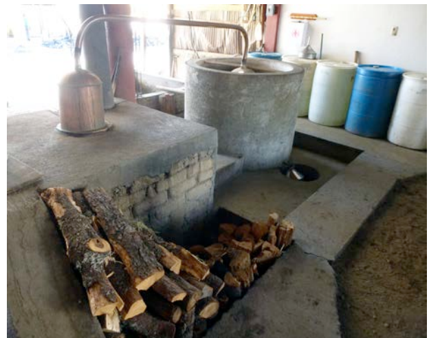
A still used to recover the alcohol from cooked agave
